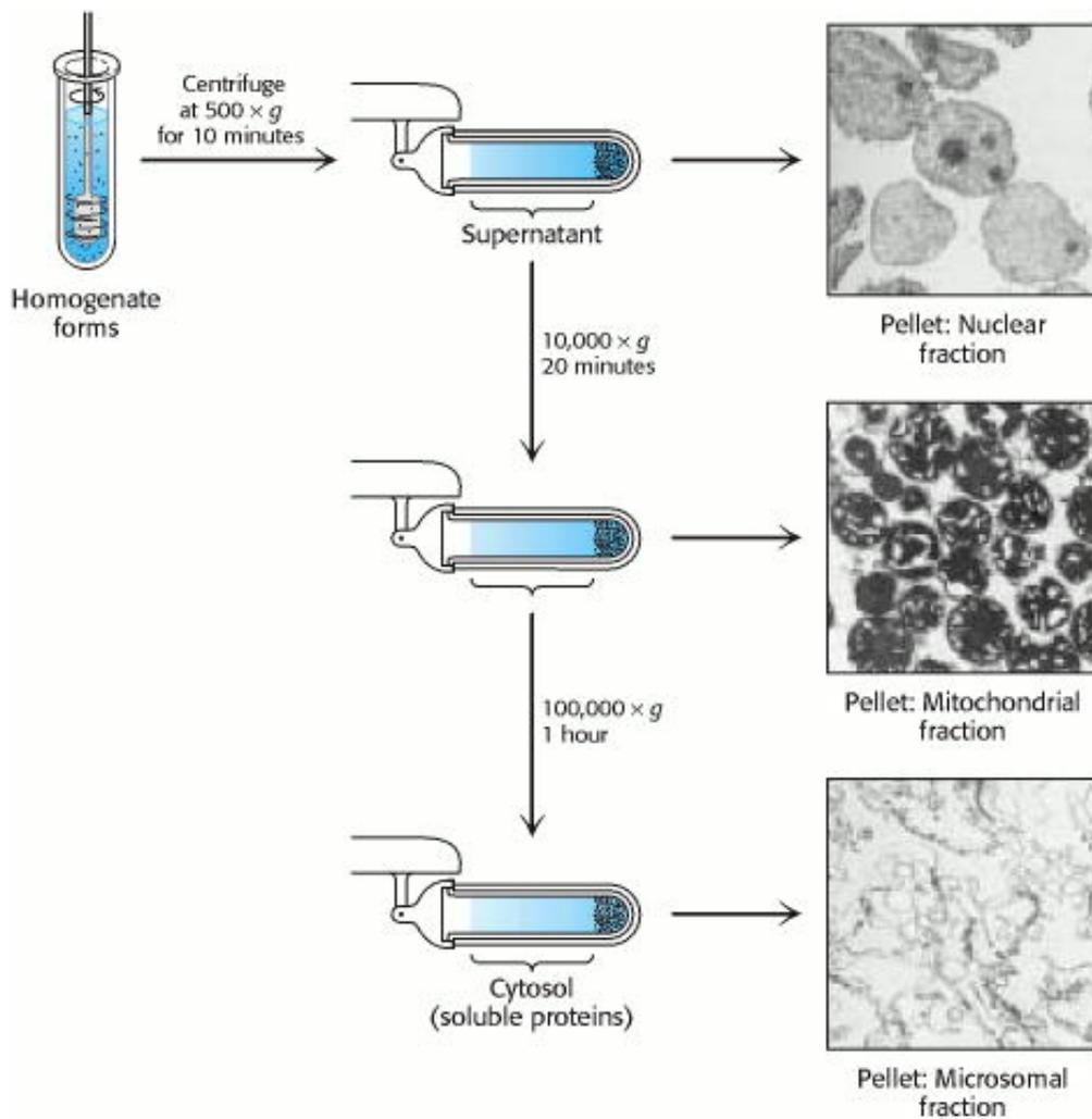
**Figure 4.1. Differential Centrifugation.** Cells are disrupted in a homogenizer and the resulting mixture, called the homogenate, is centrifuged in a step-by-step fashion of increasing centrifugal force. The denser material will form a pellet at lower centrifugal force than will the less-dense material. The isolated fractions can be used for further purification. [Photographs courtesy of S. Fleischer and B. Fleischer.]
