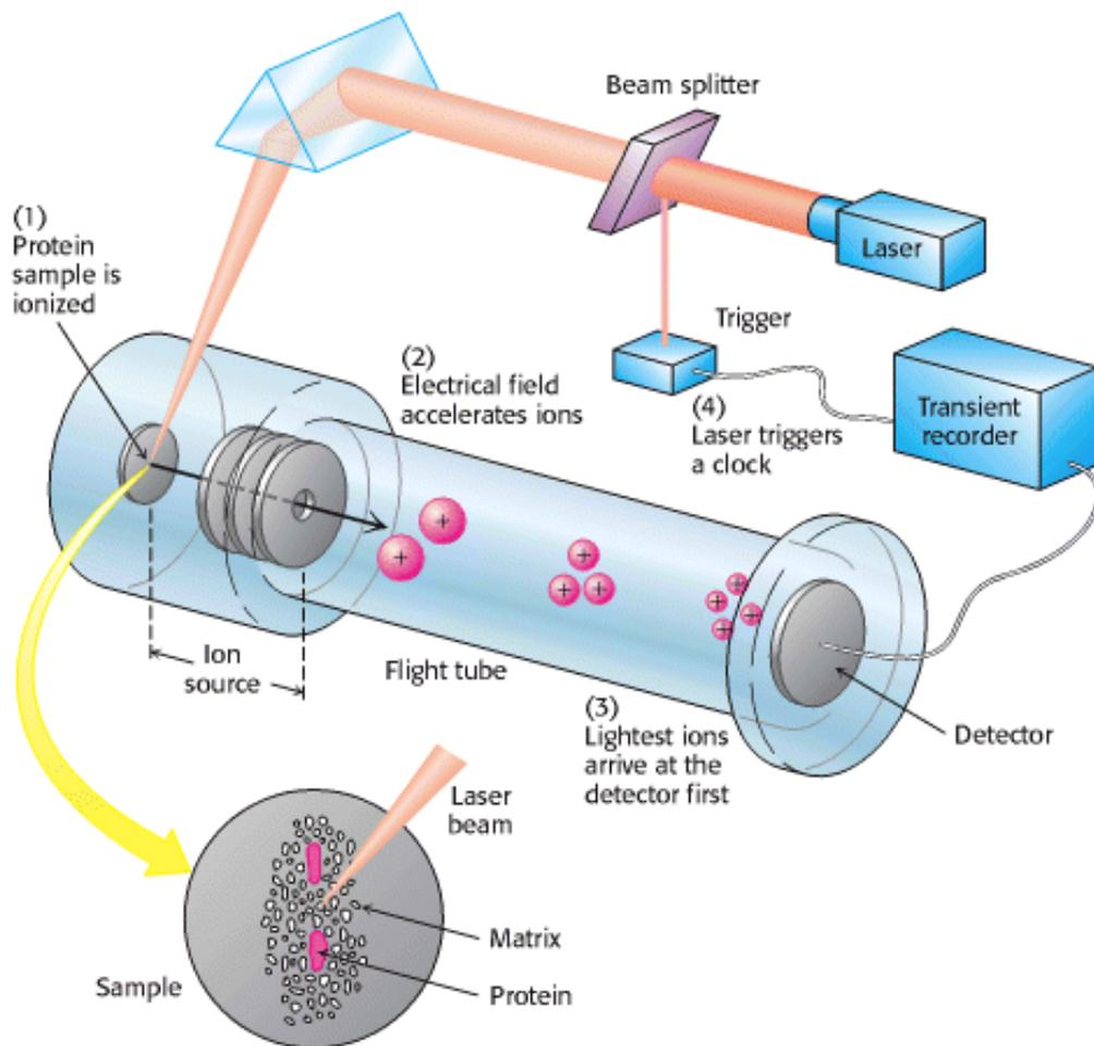
**Figure 4.16. MALDI-TOF Mass Spectrometry.** (1) The protein sample, embedded in an appropriate matrix, is ionized by the application of a laser beam. (2) An electrical field accelerates the ions formed through the flight tube toward the detector. (3) The lightest ions arrive first. (4) The ionizing laser pulse also triggers a clock that measures the time of flight (TOF) for the ions. [After J. T. Watson, *Introduction to Mass Spectrometry*, 3d ed. (Lippincott-Raven, 1997), p. 279.]
