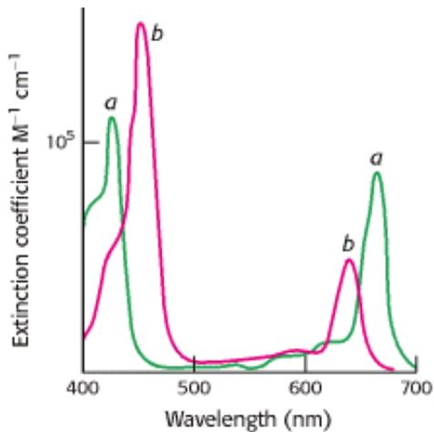
**Figure 19.29. Absorption Spectra of Chlorophyll. A and B .**
