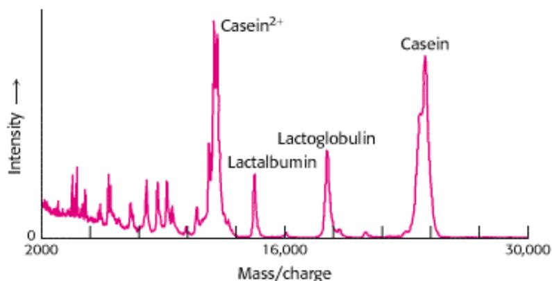
**Milk, a source of nourishment for all mammals, is composed, in part, of a variety of proteins.** The protein components of milk are revealed by the technique of MALDI-TOF mass spectrometry, which separates molecules on the basis of their mass to charge ratio. [(Left) Jean Paul Iris/FPG (Right) courtesy of Brian Chait.]
