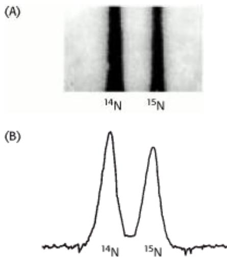
**Figure 5.14. Resolution of  $^{14}\text{N}$  DNA and  $^{15}\text{N}$  DNA by density-gradient centrifugation.** (A) Ultraviolet absorption photograph of a centrifuge cell showing the two distinct bands of DNA. (B) Densitometric tracing of the absorption photograph. [From M. Meselson and F. W. Stahl. *Proc. Natl. Acad. Sci. U.S.A.* 44(1958):671.]
