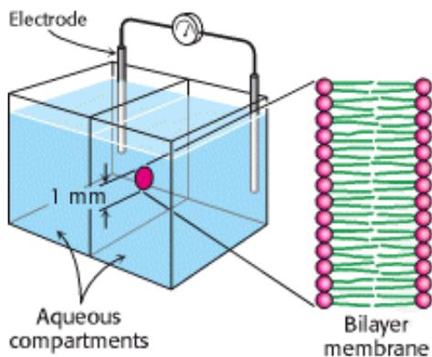
**Figure 12.14. Experimental Arrangement for the Study of Planar Bilayer Membrane.** A bilayer membrane is formed across a 1-mm hole in a septum that separates two aqueous compartments. This arrangement permits measurements of the permeability and electrical conductance of lipid bilayers.
