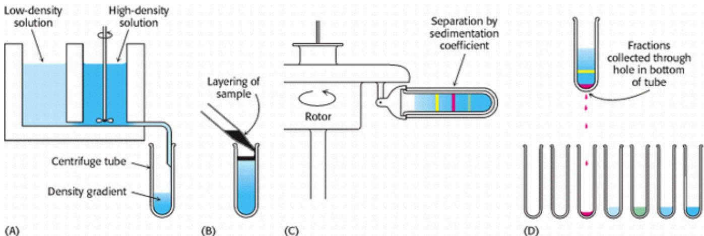
**Figure 4.15. Zonal Centrifugation.** The steps are as follows: (A) form a density gradient, (B) layer the sample on top of the gradient, (C) place the tube in a swinging-bucket rotor and centrifuge it, and (D) collect the samples. [After D. Freifelder, *Physical Biochemistry*, 2d ed. (W. H. Freeman and Company, 1982), p. 397.]
