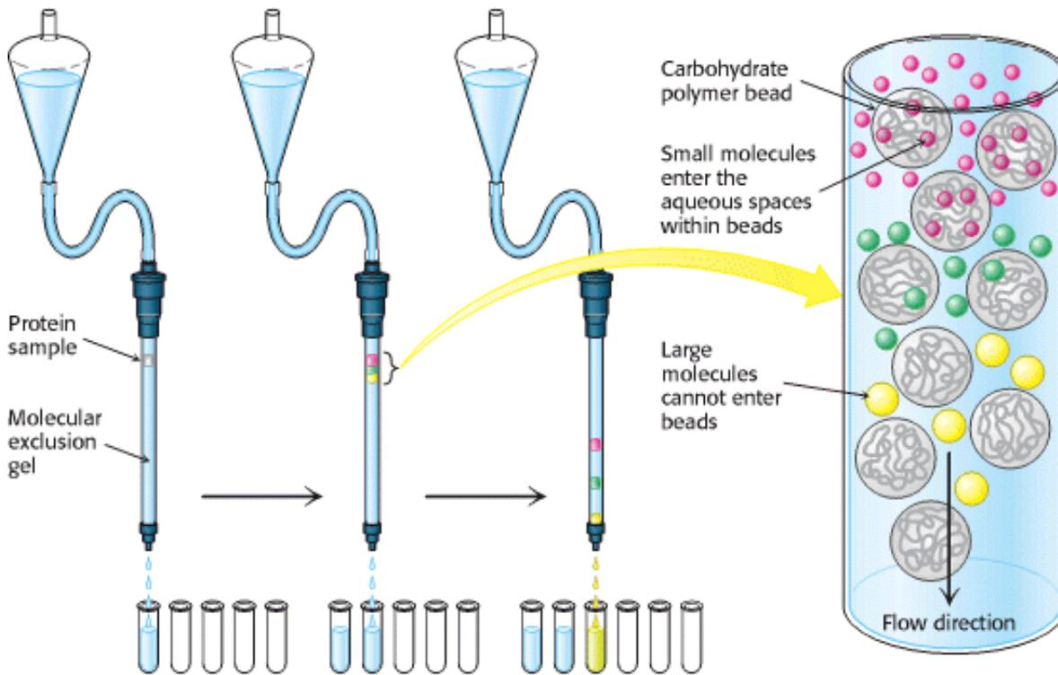
**Figure 4.3. Gel Filtration Chromatography.** A mixture of proteins in a small volume is applied to a column filled with porous beads. Because large proteins cannot enter the internal volume of the beads, they emerge sooner than do small ones.
